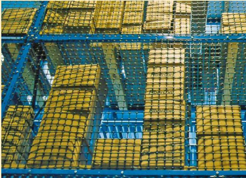
Industrial Netting’s Rack Guard System protects warehouse workers from falling objects.
