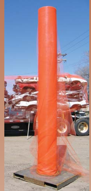
14 foot wide roll mounted on "lazy susan" adapted for front loader.
