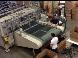
Industrial Netting offers customers a variety of custom converting solutions including custom sheeting, precision slitting, die cutting and sonic welding. While tolerances can vary with mesh configuration,  $\pm 0.030$ " is achievable for most custom cuts. For a full range of value added services visit <a href="https://www.industrialnetting.com/services">www.industrialnetting.com/services</a> or call 800-328-8456 to speak with a representative.
